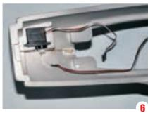
Picture 3:a Servo with 250mm Wire is Required for Pilot Ejection Function
